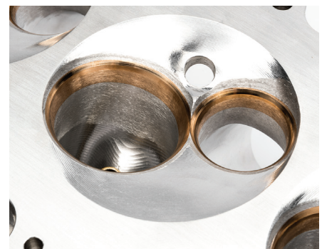
CNC LS combustion chamber & ports complete with 50° valve job, blended alloy valve seats for N 2 O & high boost applications.
